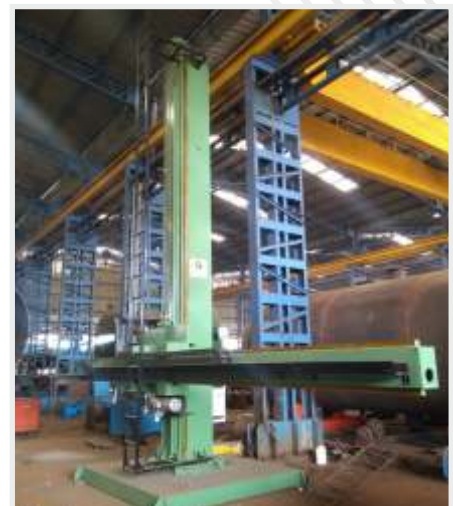
Welding Column & Boom
