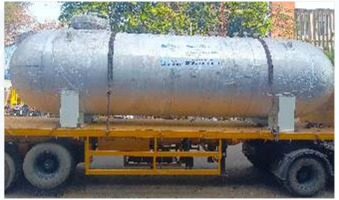
30M 3 Liquid Ammonia Vessels for Adani Project
