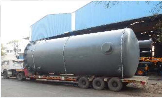
4 mtr. Dia & 12 mtr. Length Vessels For Steel Plant
