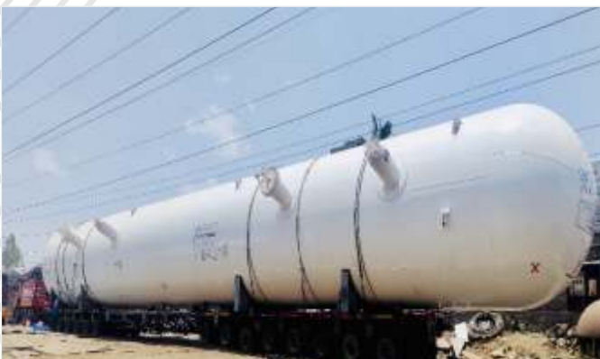
2nos 577m 3 Propane Mounded Vessels
