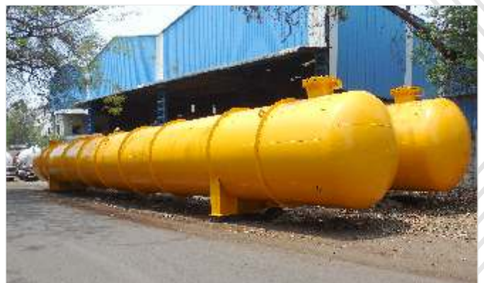
252M 3 Ammonia Storage Vessels for Harman Finnochem Ltd.
