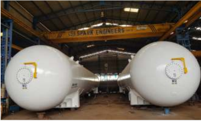
477m 3 LPG Storage Vessels - Exported to Fiji Island
