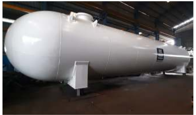
232M 3 Ammonia Storage Vessels for SVJL Project
