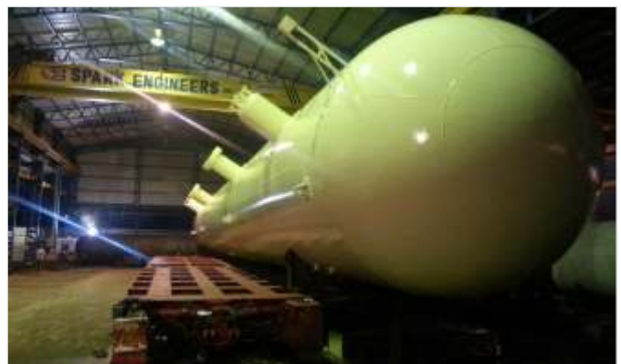
2nos x 545m 3 Propane Mounded Vessels Size : 4.5mtr Dia x 40 Mtr long x 125 ton weight
