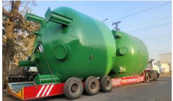
93 Nos of Sand Filters Supplied to Jindal Steel, Plant Size: 5 Mtr Dia x 8mtr long, wt. 20 ton
